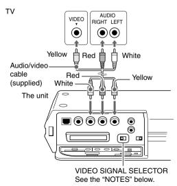
This illustration is upside down. (The bottom side is up.) For details on the connectors' name, see page 38.
